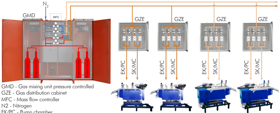
Schematic overview gas distribution cabinet GZE
